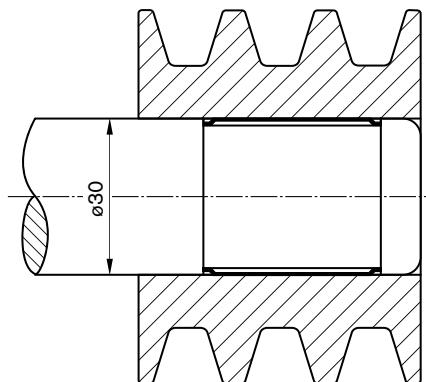
This figure shows a V-belt pulley fastened to a shaft by means of a tolerance ring 0820-030-08. The connection transfers a torque M of at least 88 Nm.
