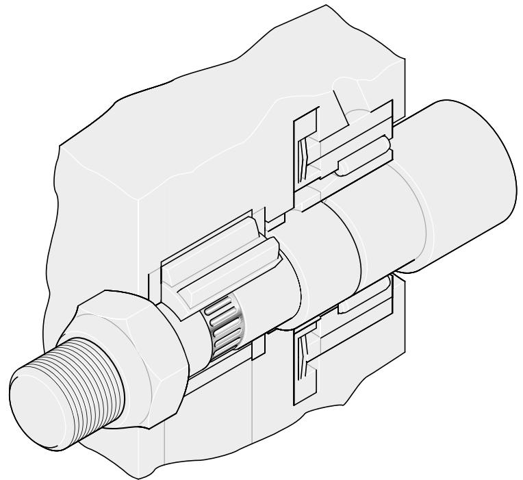
Pinion fastening with Rexroth tolerance ring in turbomolecular pumps.
