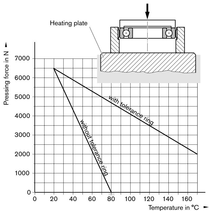
The graph shows the mounting of rolling bearings of 200 mm diameter at a temperature of 20°C with and without a tolerance ring. In both cases the pressing force is initially 6500 N. As the temperature rises, the pressing force falls. For rolling bearings mounted without a tolerance ring, the pressing force falls to zero at a temperature of 80°C, whereas with a tolerance ring there is still a small pressure force of 2000 N at a temperature of 170°C.
