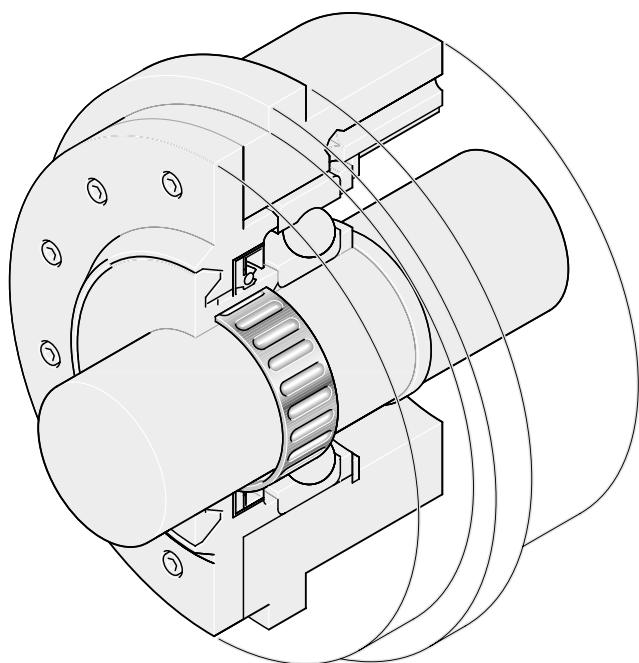
Fastening of a labyrinth ring on a shaft using a Rexroth tolerance ring
