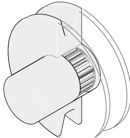
Fastening of a V-belt pulley on a shaft (instead of a contour-locking joint with keyway).
