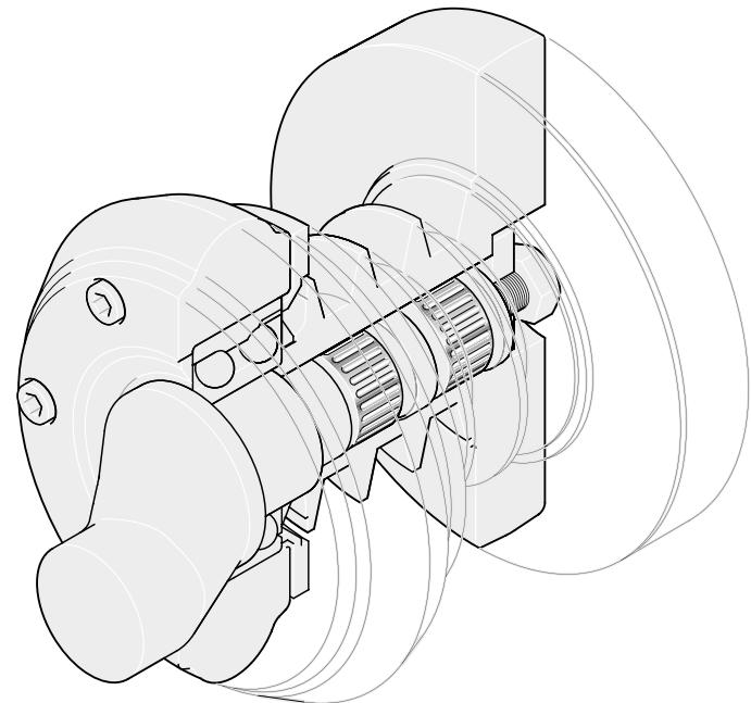
Tandem mounting of Rexroth tolerance rings in a mowing machine drive.
