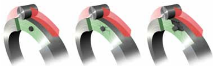
Formation of damage below the surface
