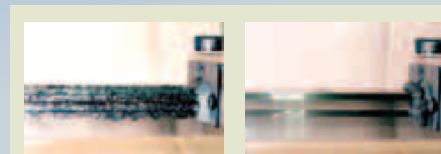
Before passage of ball slide (Significant foreign matter remains after passage of the slider)
